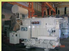
Furnace Transformer [Oil Forced Water Cooled]
